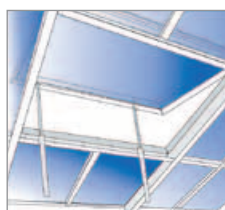
3 Roof window opening outwards at bottom Tandem with linear drive units
