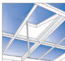
1 Top hung opening outwards at bottom With linear drive unit
