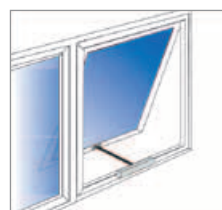
4 Top hung opening outwards at bottom With chain drive unit
