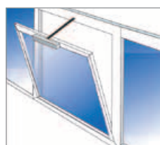
17 Bottom hung opening inwards at top With chain drive unit
