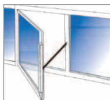
11 Side hung opening inwards With chain drive unit
