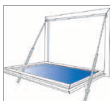
18 Bottom hung opening inwards at top Tandem with linear drive unit
