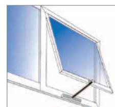
5 Top hung opening inwards at bottom With chain drive unit
